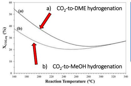
Due to methanol consumption by dehydration reaction, the one-step process is more efficient than the two-step process, with a main benefit at low temperature and high pressure.
