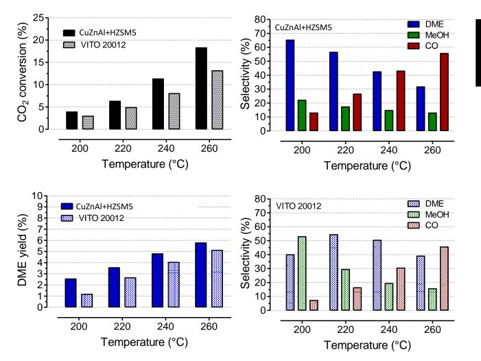
Conventional catalyst exhibits a better performance than the 3D printed crushed monolith
