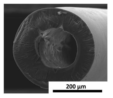
Maximum take up rate: 20 m/min OD/ID: 370 μm / 160 μm
