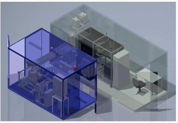
Layouts of compressor (left) and electrolyser (right) containers
