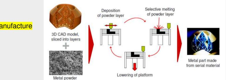
Reactor manufacture Selective Laser Melting
