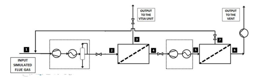
The two-stage membrane section has been tested successfully according to work programme using polyimide commercial membranes
