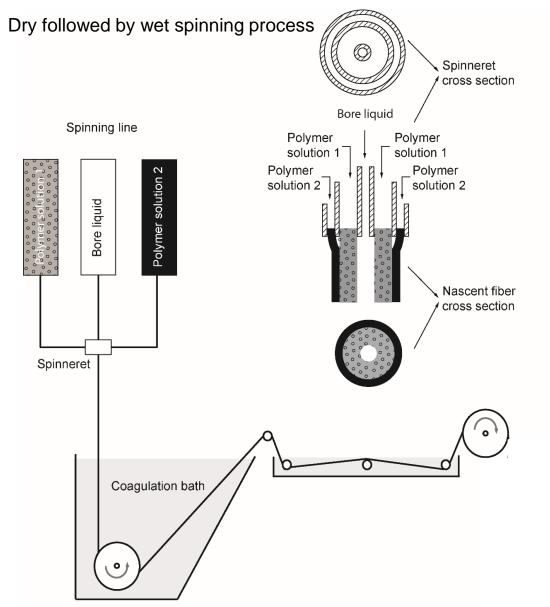
**Process parameters Dope Composition** Dope Flow rate **Bore Composition Bore Flow Rate** Spinning Temp **Coagulation Bath Temp** Air Gap height Take-up rate Room T Humidity
