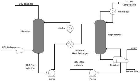
Figure 2. Typical flowsheet of a basic chemical absorption process for CO<sub>2</sub> capture.
