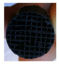
Furnace drying at 40°C Channel diameter 1.4 mm Wall thickness 0.6 mm
