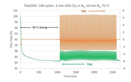
High selectivity to CO2 over other gases as well as stable performance over high number of sorption/desorption cycles.
