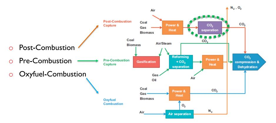
Figure 1. Schematic conceptual representation of CO<sub>2</sub> capture technologies [12].
