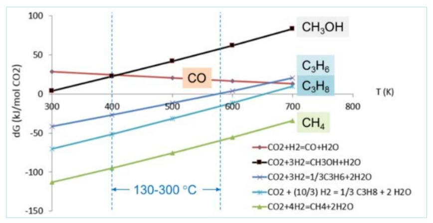
**Gibbs free energy vs. Temperature for CO<sub>2</sub> hydrogenation reactions**
