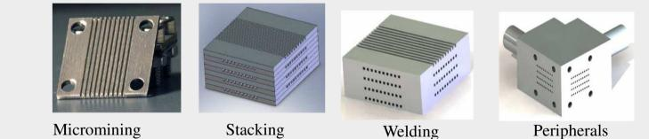
Stages needed for the manufacture of microreactors. Adapted from *S. Cruz et al. (2011). Chemical Engineering Journal 167. 634-642*
