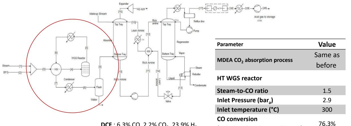
**DCF** : 6.3% CO, 2.2% CO<sub>2</sub>, 23.9% H<sub>2</sub>, 61.8% N<sub>2</sub>, 5.5% H<sub>2</sub>O
