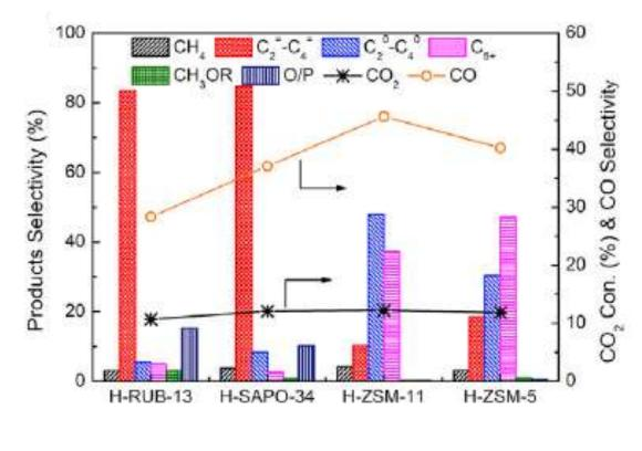
$Zn_{0.5}Ce_{0.2}Zr_{1.8}O_4$  + zeolite, 350 °C, 10 bar, H<sub>2</sub>/CO<sub>2</sub> = 3:1, GHSV = 4,800 mL/gh
