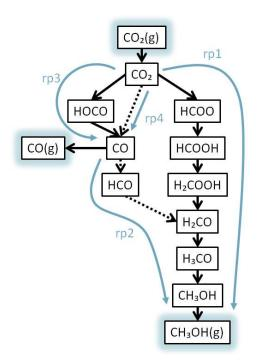
Overall reaction scheme. Black arrows represent the elementary reaction steps and blue arrows the reaction pathways. Reaction species in black squares without "(g)" are adsorbed on the catalyst's surface.
