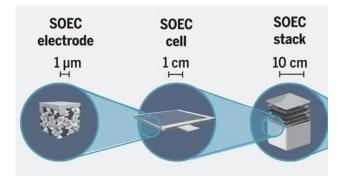
SOEC: Solid oxide electrolyte cells
