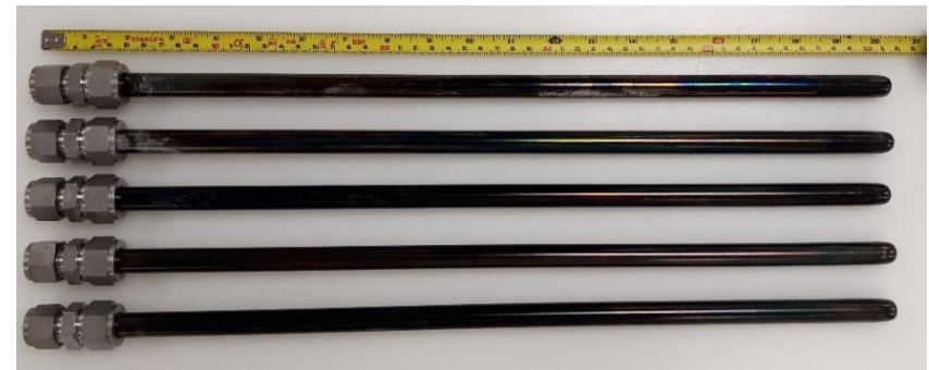
Ceramic supported thin double skin Pd-based membranes prepared for the prototype
