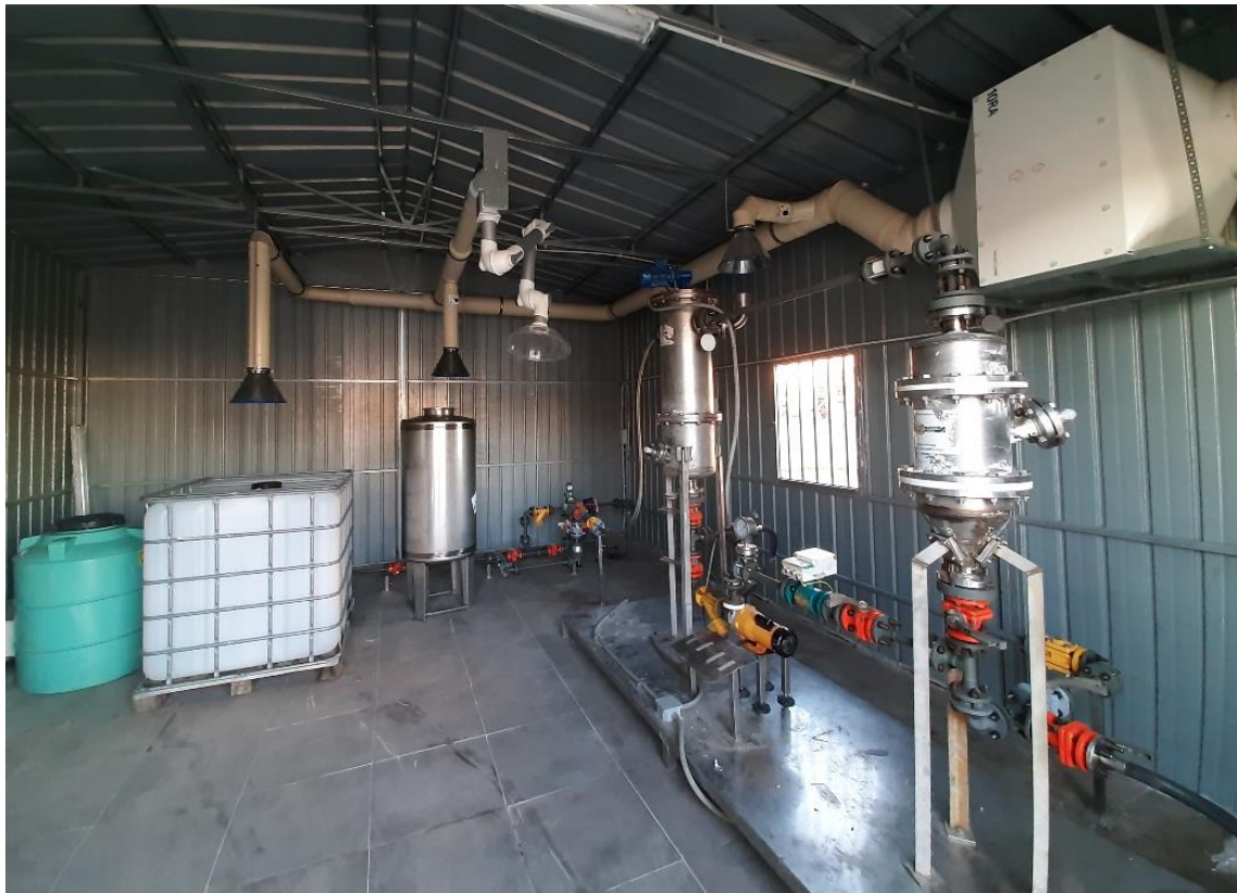
Eco Recycling's pilot plant for the metallic and ceramic membrane recycling process.
