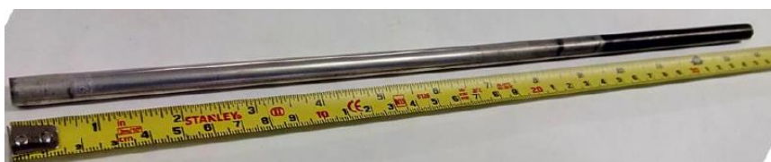
Figure 6. Metallic-supported Pd-based membranes. Reproduced with permission from TECNALIA.
