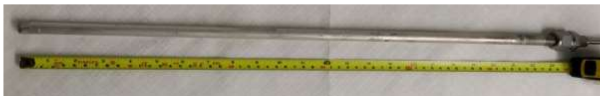
Figure 7. Thin Pd-based membrane onto 50 cm long porous metallic support
