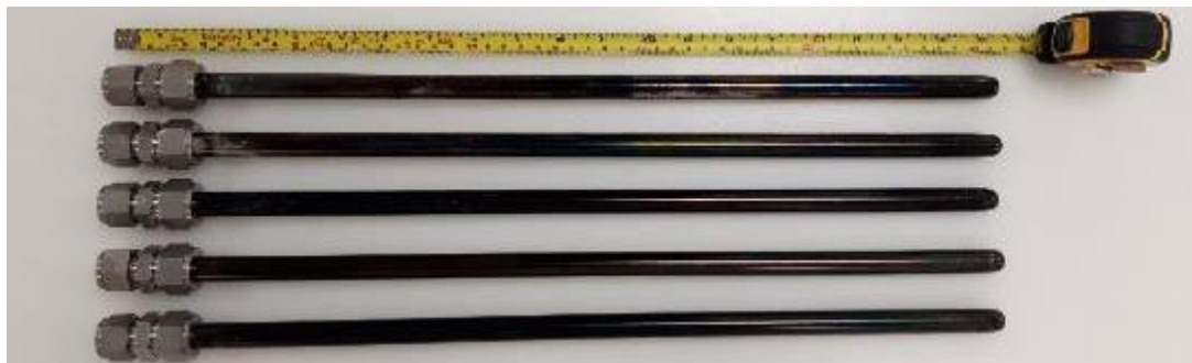
Figure 9. Ceramic supported thin double skin Pd-based membranes prepared for the MA-SER prototype.
