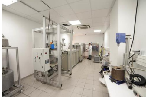
Figure 8. Pilot plant for scaling-up the production of HF MMMs: pre-combustion CO 2 capture (left) and post-combustion CO 2 capture (right).
